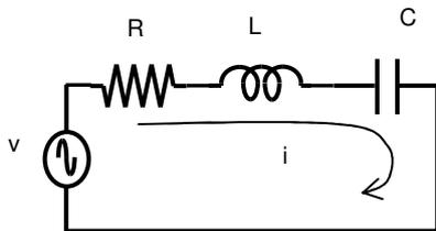
$$v = iR + iZ_L + iZ_C = i \left( R + j\omega L + \frac{1}{j\omega C} \right).$$
