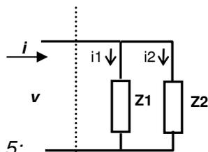
$$i = i_1 + i_2 = \frac{v}{Z_1} + \frac{v}{Z_2} \quad \therefore \frac{i}{v} = \frac{1}{Z} = \frac{1}{Z_1} + \frac{1}{Z_2}$$
