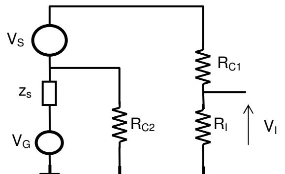
$$V_{IS} = V_s \cdot \frac{R_I}{(Z_s // R_{C2}) + R_{C1} + R_I}$$
