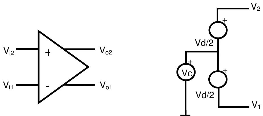
$$V_d = V_2 - V_1 \quad ; \quad V_c = \frac{V_2 + V_1}{2}$$
