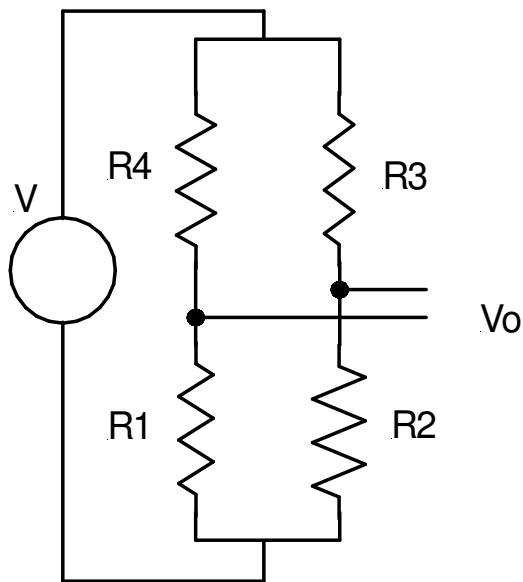
$$V_o = \left( \frac{R_2}{R_2 + R_3} - \frac{R_1}{R_1 + R_4} \right) V = \\ = \frac{\frac{R_4}{R_1} - \frac{R_3}{R_2}}{\left(1 + \frac{R_4}{R_1}\right)\left(1 + \frac{R_3}{R_2}\right)} V$$
